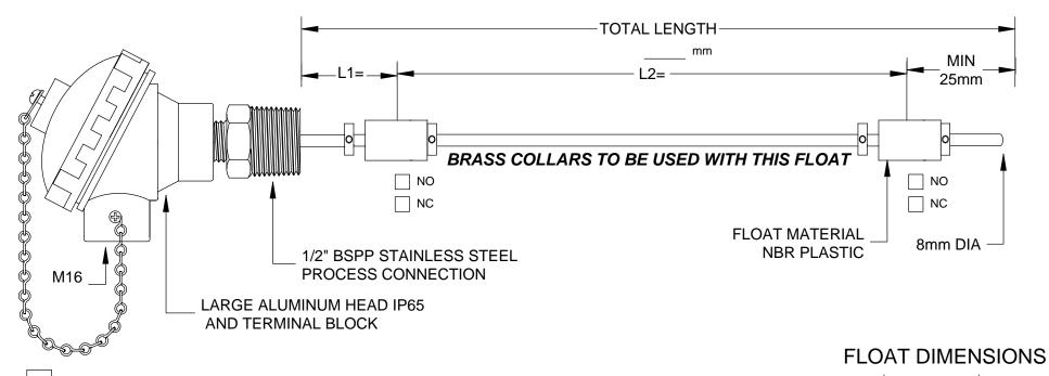
STANDARD - NO or NC CONTACT RATED AT 32V AC/DC @ 500mA RESISTIVE LOAD
